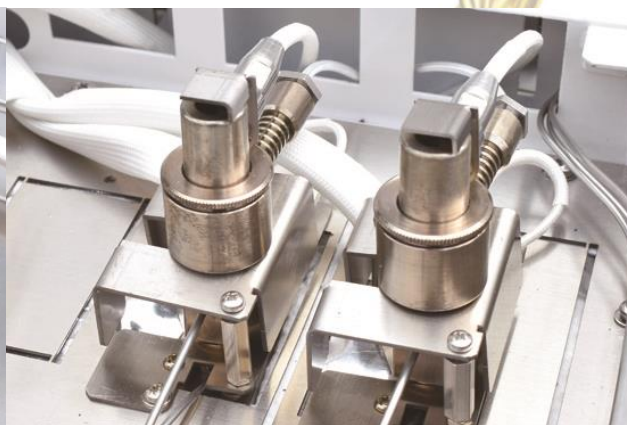
FID(High sensitivity and low noise)
